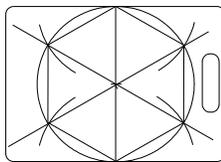
While cutting the hub using a saber saw, I learned that this must be done at low speed or the cut will try to weld back together from the heat generated in the blade by friction.
