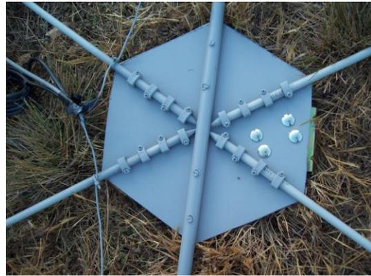
Impedance matching is accomplished with a delta match of automotive wire adjusted by "cut and try" with an SWR bridge and a transceiver set to low power. The delta match is fed with a half wave coaxial balun.
