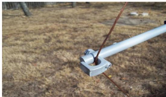
The length of the driven element was calculated using the formula  $\text{Length} = 468/\text{Frequency}$  (50.125 MHz) or 9.34 feet.
