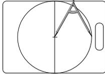
Without changing the setting of the compass, I drew a short arc either side of the line where it intersected the circle on both sides of the board.
